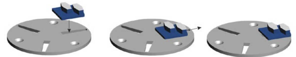
Figure 4-4 How to fit the diamond tools on the Scan-On plate
