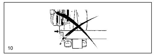
4.6.2 Cutting blades are only designed to cut materials on their edges. Never use the side surfaces for grinding purposes as this can break the disc! (10).
