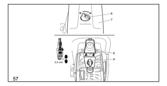
Turn the cover lock (6) to the "unlocked " position and carefully remove the filter cover (7).
