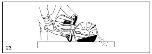
The quick rotation of the cutting blade at the contact point tears the material and throws it out of the cutting groove. As far from the cut as possible (behind it), swivel the protective hood down (23) to divert the workpiece particles that have been cut away from the operator.
