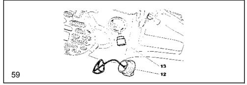
The felt filter (13) of the suction head can become clogged during operation. To ensure an unrestricted flow of fuel to the carburetor, the suction head should be replaced about every 3 months.
