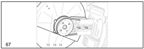
Press the cutting attachment (13) to the outer position against the gear arm receptacle.
