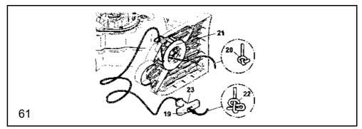
Feed in new rope with a diameter of 4.0 mm (0.16") and a length of 1,000 mm (40"), as in the illustration (do not forget the disc (19)) and knot both ends.
