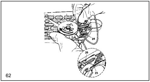
Pass the rope through the recess (24) on the rope drum and, together with the rope, turn the rope drum twice in the direction of the arrow.
