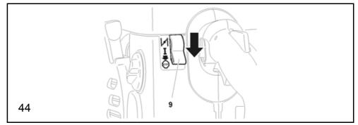
Press the multifunction switch (9) down to the "Stop" position.
