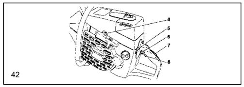
Press the multifunction switch (5) upward (choke position).
