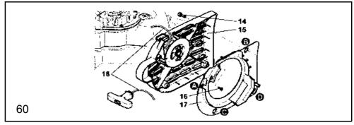
Release the four screws (14). Remove the valve housing (15).
