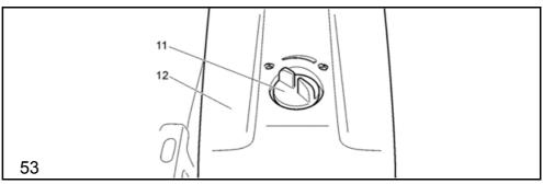
Turn the cover lock (11) to the "unlocked  $^{\bigcirc}$ " position and carefully remove the filter cover (12).
