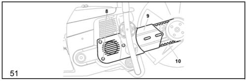
Loosen the screws (8) and take off the crankcase cover (9).
