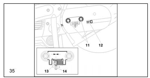
**NOTE:** To tighten the V-belt and to check the tension, you must loosen both mounting nuts (**11**).
