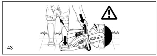
Put your hand around the bow handle grip and hold it firmly while you press the cut-off saw against the ground.
