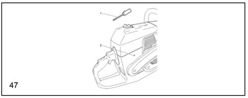
Set the speed for the idle position with the screwdriver that was included in delivery.
