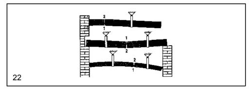
4.10.10 Always notch material that is under tension (material that is supported or embedded in a wall) on the pressure face and then cut from the opposite side so that the cutting blade does not get pinched (22). **Secure the material that is to be cut so that it does not fall!**
