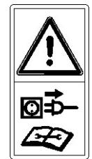
Warning: Before carrying out any maintenance operation described in this manual, disconnect the plug of the machine.
