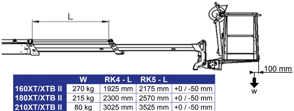
The red warning light for overloading will illuminate as soon as the **RK4** has stopped the movement. While at the outreach limit, the red warning light and the green signal light will flash in turns. In this situation, the lift can be operated in the direction, in which it remains inside the permitted outreach area.
