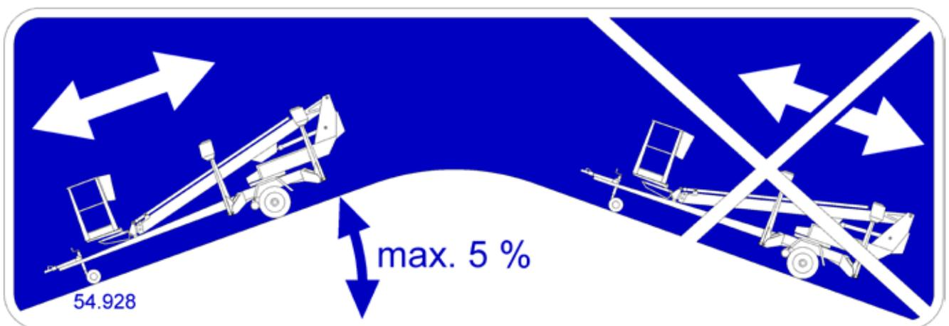
**Do not drive downhill with the driving device, if the inclination of the surface is more than 5 per cent, i.e., more than 1/20 (corresponding to a descent of 0.5 m over a distance of 10 m). If the gradient of the surface is greater than this, you may lose control of the device.**
