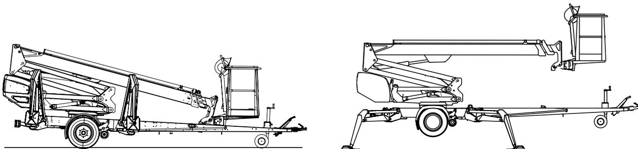
The primary power source of the lift is electric motor. The outriggers and the boom system are hydraulically powered.
