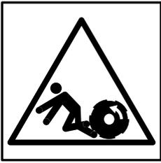
Crush hazard - moving parts
