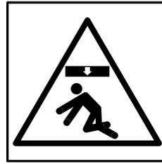
Crush hazard - falling objects
