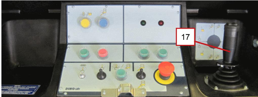
The functions to be controlled are selected using the "dead-man-buttons" at the end of the joystick. Always press the button first, and only after that, turn the handle. The safety connection prevents the movements, if the handle is turned before depressing the button.
