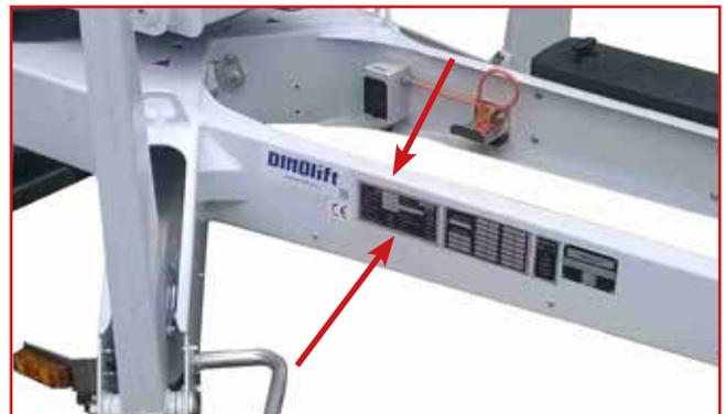
The nameplate of the trailer is located on the tow-bar, on the right-hand side of the nameplate of the lift, as shown in the picture.
