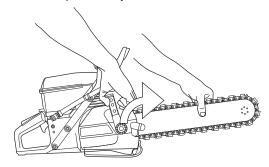
Lock the chain tension by tightening the counter screw.
