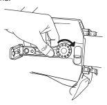
Release the spring. Hold the bar upwards as you move the handle forward. Note that the arm's mechanical stop shall not be reached. The stop prevents the arm from pointing forwards and prevents cutting.
