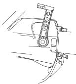
Move the lever to its rear, lower position. Push in the spring on the chain tensioner handle and turn the bar nut clockwise by hand
