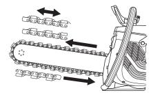
When using a chain with double rakers, the chain can be fitted either way round. When using a chain with one raker, the chain should always be fitted the right way round. The raker should guide the segment at the right height in the cut.
