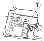
Rec. idle speed: 2700 rpm
