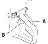
The trigger lock remains pressed in as long as the throttle is pressed. When the grip on the handle is released the throttle trigger and the throttle trigger lock both return to their original positions. This is controlled by two independent return spring systems. This means that the throttle trigger is automatically locked in the idle position.
