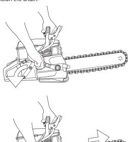
Hold the bar upwards as you move the handle forward.
