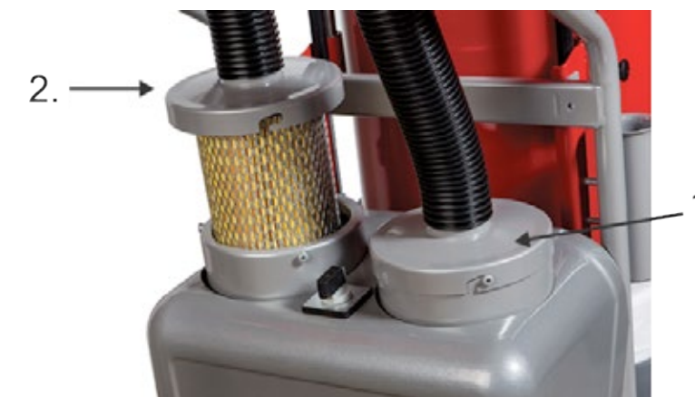
Figure 7 Top of the HEPA filter Scan Dust 2900
