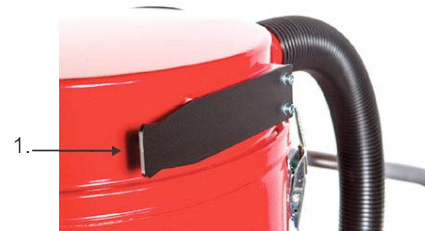
Figure 3 Scan Dust 2900 Filter cleaning
