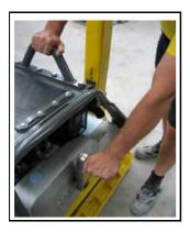
5. Grab the crank handle with one hand. Support yourself on the protective cage with the other hand.
