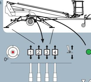
NOTE! The support outriggers cannot be moved when the boom is not on its support.
