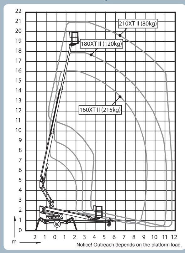
160XT || 160XTB || 180XT || 180XTB || 210XT || 210XTB || 1990 kg 2175 kg 2300 kg 2390 kg 2465 kg 2590 kg Weight Transport height 2,30 m 2,30 m 2,33 m Transport width 1.80 m 1.95 m 1.95 m Support width 3,9 / 4,3 m 3,9 / 4,2 m 3,9 / 4,3 m Lifting capacity 215 kg 215 kg 215 kg
